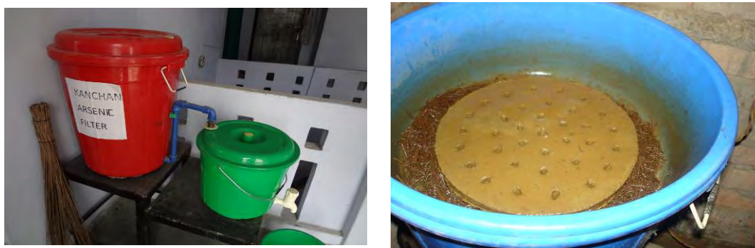
Photo.6.4 Using filtering system for arsenic removal in houses in Parasi.
