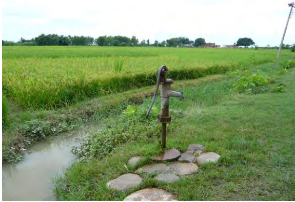
1. A tube-well of Khokharpuruwa recorded the highest value of the arsenic concentration, 1,048ppb (Photo: September 2009)
